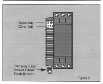
The Model MC60V P/I Transmitter is a solid state pressure to electrical converter that translates a pneumatic (pressure) signal into a 4-20 mA two wire output signal. Span and zero calibration adjustments are easily accessible through the front of the case. The 4-20 mA loop can be monitored at the test terminals without disconnecting the MC60 or creating a special hookup.
