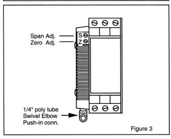
The Model MC60 P/I Transmitter is a solid state pressure to electrical converter that translates a pneumatic (pressure) signal into a 4-20 mA two wire output signal. Span and zero calibration adjustments are easily accessible through the front of the case. The 4-20 mA loop can be monitored at the test terminals without disconnecting the MC60 or creating a special hookup.
