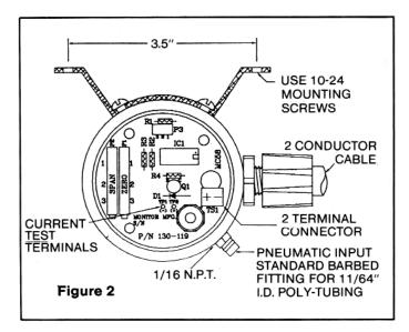
The Model MC58 P/I Transmitter is a solid state pressure to electrical converter that translates a pneumatic (pressure) signal into a 4-20 mA two wire output signal. Span and zero calibration adjustments are easily accessible from the front of the unit when the cover is removed. The 4-20 mA loop can be monitored at the test terminals on the PC board without disconnecting the MC58 or creating a special hookup.
